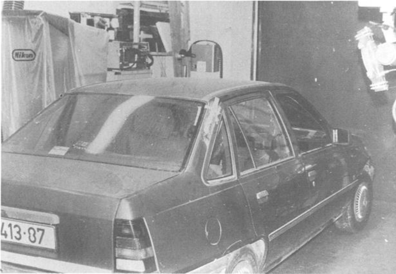
FIG. 1—Suspected vehicle in X-ray examination room; note X-ray tube positioned in upper-right hand corner.
